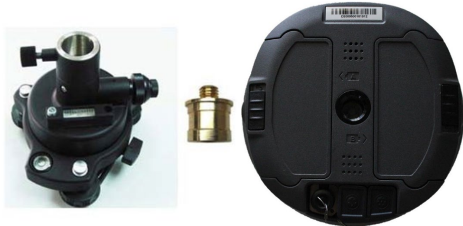
Figure 2-6: Installing S631 on a tribrach
