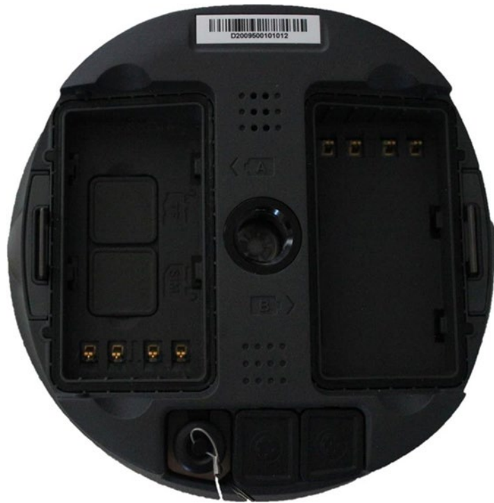
Figure 2-12: SD card/SIM card slot
