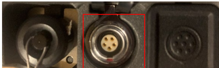
Figure 2-9: External power connector
