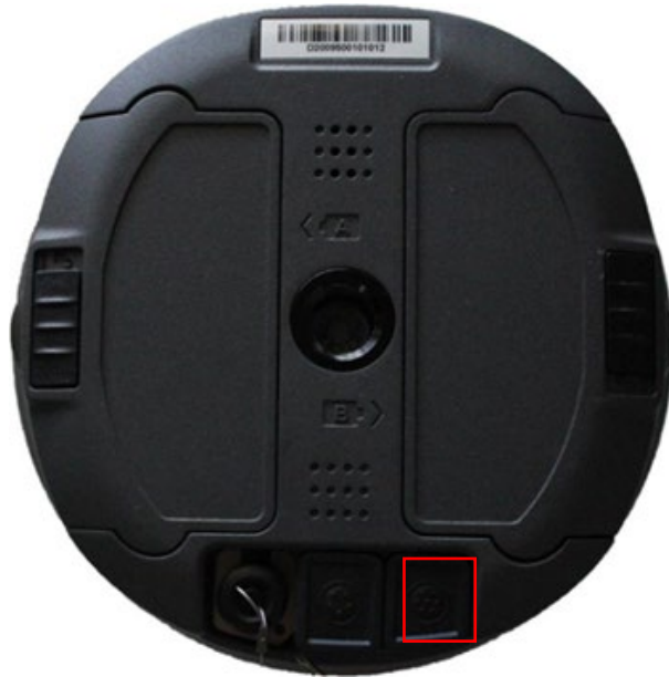
Figure 2-10: 7-pin diagnostic connector
