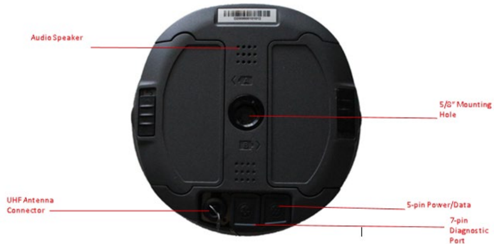
Figure 2-1: S631 ports and connectors
