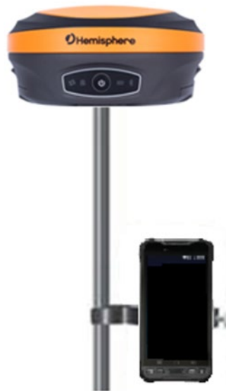
Figure 2-8: Range pole installation
